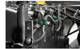
Coil-on -plug: Low maintenance & efficient electrical system High uptime with easy fault diagnosis system
